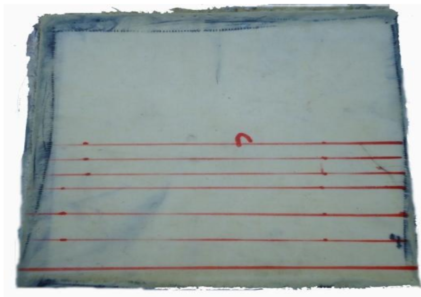
Fig. 01 Glass fiber reinforced polyurethane resin composite sheet
